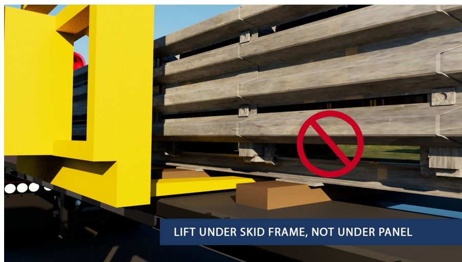
Figure 7a: Lift Below the Skid Frame
