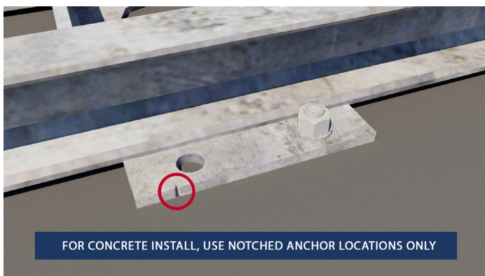
Figure 9: Concrete Anchor Locations are Notched
